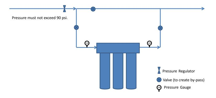
If you experience a drop in household pressure check these gauges. A large pressure drop (compared to new) will indicate the sediment filter is clogged and should be replaced.
